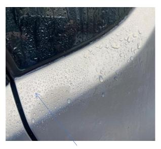
Strong hydrophobicity on the coated section.
