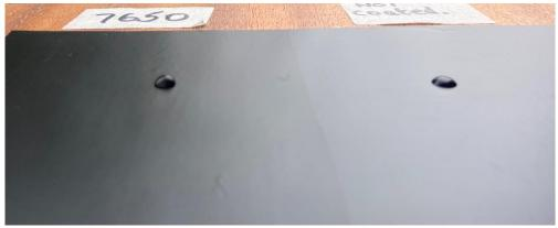
Vinyl wraps are inherently hydrophobic. These images show that the 7650 coating significantly enhances the hydrophobicity of the vinyl.
