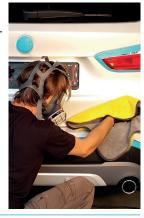
In warm conditions the coating becomes dust dry after 2 hours and touch dry after 5 hours. After this, the coating will be dry enough that you may use the vehicle again but the coating is still far from being fully cured and so avoid brushing against the surface with bags or keys.
