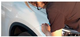
After completion of the general cleaning process, deep clean the surface with alcohol (e.g. at least 70% isopropyl or ethanol alcohol), so that all contaminants are removed from the surface. The use of a clay bar cleaning process is also suitable. The simple message is that the coating should only be applied to surfaces which are free of contamination.
